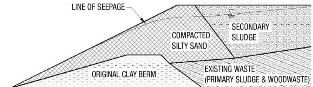
**Figure 1.** Cross section of the berm shown in Photo 1.
