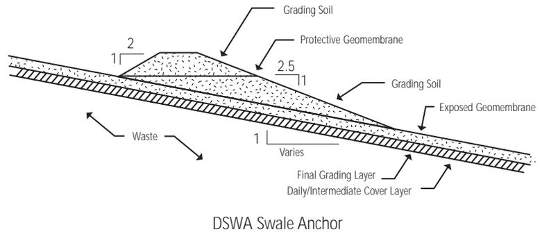
**Figure 5a:** Detail of swale bench anchor used at the Delaware Solid Waste Authority EGC project.
