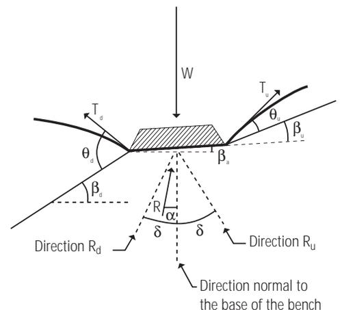
**Figure 2:** Forces acting on an anchor bench when the geomembrane is uplifted by wind action.
