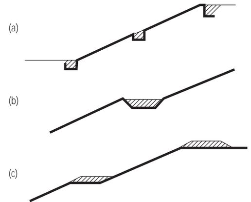
**Figure 1:** Examples of anchor trenches (*a*, *b*) and a bench (*c*).
