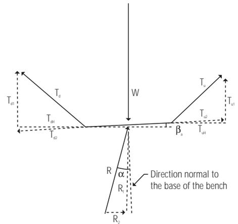
**Figure 3:** Decomposition of the forces acting on an anchor bench into vertical components (subscript 1) and components parallel to the base of the anchor bench (subscript 2).
