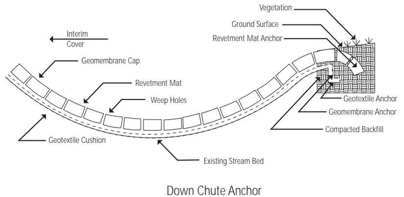
**Figure 6:** Section of a drainage down-chute.
