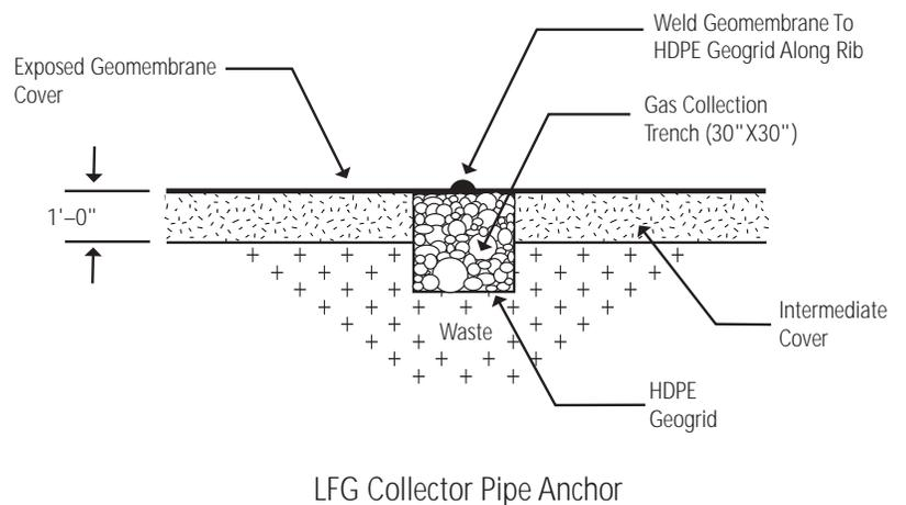
**Figure 7:** Restraint of EGC by attachment to LFG collection trenches.
