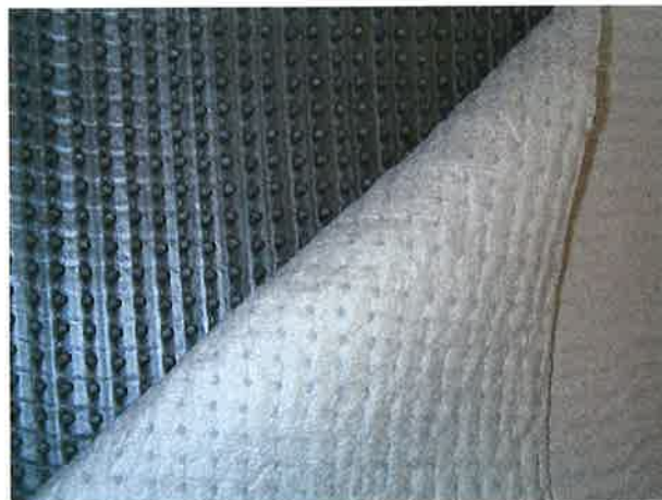
Figure 2(b) Landfill final cover composite – a close look
